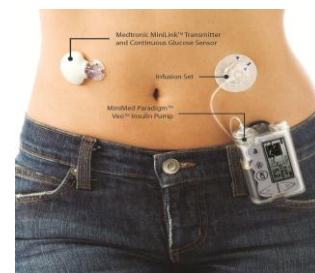
CGM data sent via wireless transmitter to an insulin pump
